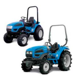
From the smallest 1-25 to the largest 1-35, all models in this range are specially designed to perform light farm tasks as well as lawn and landscape maintenance jobs. They are powered by Tier 3-compliant, 3-cylinder, water-cooled diesel engines delivering 22, 28 and 34 hp, respectively.
